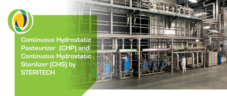
Our systems Continuous Hydrostatic Pasteurizer (CHP) and Continuous Hydrostatic Sterilizer (CHS) include 3 sections: 1st section for temperature build-up, a central section for heat treatment, and a 3rd section for cooling. Each area is further subdivided into several columns, in which specific temperature and pressure levels can be set separately\*.
