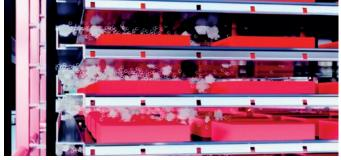
These nozzles are fed by a pump which recovers water at the bottom of each section, maintains it at the desired temperature through heat exchange, and forwards it to the spray nozzles. Water is then recycled on a continuous basis.
